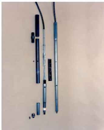
Laser Induced Fluorescence Sensor Thermal Desorption Petroleum (POL) Sensor VOC Hybrid Sensor/Sampler Electro-Chemical Explosives (TNT, HMX, RDX) Sensor
