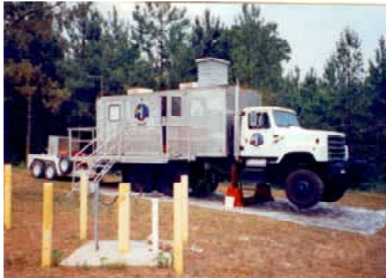
SCAPS Truck Conducting Characterization Acquisition of Subsurface Soil Layering and Contamination Processing
