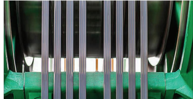
UltraRope in the elevator hoisting machine
