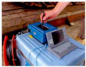
PAL-R receives signals from sensors. Field operation is minimal, and done by touching screen with special pen, Laptop is optional.
