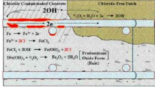
Potential Difference Between Patch and Chloride Contaminated Concrete Results in Accelerated Corrosion
