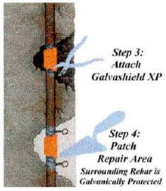
Galvashield XP Anodes Installed Prior to Patch Repair Completion
