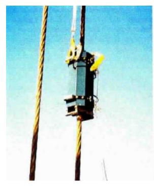
Figure 2. Test Instrument Installed on Suspender Rope
