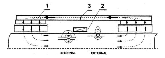
The principle of magnetic flux leakage inspection of wire rope Figure 1. 1. Magnetic Circuit
