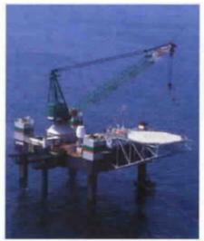
The IB909 jack-up barge returned to Massachusetts Bay to install a caisson and a ventilation pipe in order to bring air into the effluent outfall tunnel.
