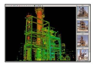
Figure 2 - Laser Scans of Construction Area
