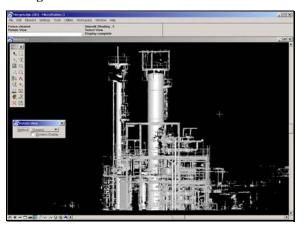
Figure 4 - Surface Model Imported into CAD to be used for clash detection on a construction project (Example is Microstation in this figure)
