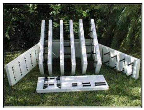
Figure 1. This picture displays the versatility and flexibility of the ECO-Block ICF building system. All three sizes are shown: 4 inch (102 mm), 6 inch (152 mm), and 8 inch (203 mm). On left is the standard side panel; on right is the standard side panel with connectors attached.
