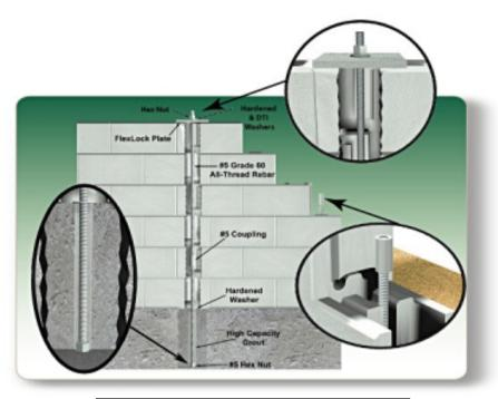
Post-Tensioning Technology Revealed
