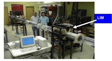
Figure 4. Testing a LIM-powered PCP at University of Misso
