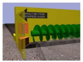
This diagram shows the asphalt feeding from the paver, with the auger crossfeeding the asphalt out to the Shoulder Wedge Maker™, then compacting the asphalt and creating a wedge along the edge of the roadway. The Shoulder Wedge Maker™ creates a smooth wedge for easy transition onto the roadway if a vehicle were to veer from the road.
