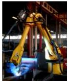
Left: Robotic welding of the outer collar to the wide flange beam takes place in the factory resulting in superior weld quality accomplished in a fraction of the time when compared to field welding.
