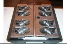
Left: close-up of outer collar plate that is machined to .006 in. - and then robotically welded (in the plant) to the end of a wide flange beam.
