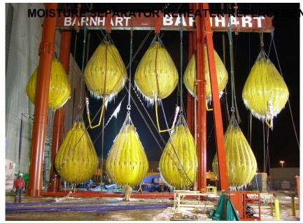
Testing modular lift tower with water weights
