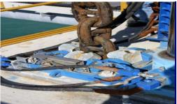
**Chain Locks on Ramp Hoisting Mechanism**
