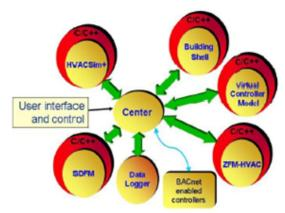
A representation of the various software components of the VCBT. Included are models which simulate the rooms and HVAC systems in a building, smoke and heat sensors, fire and smoke distribution, and a virtual controller model (to enable emulation of very large buildings). The Center component manages all communications and data transfer between the component models.
