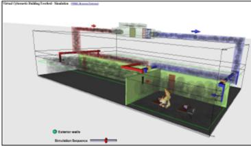
VRML representation of the VCBT showing smoke and heat migration through the building and HVAC equipment, using a 2 layer fire model.
