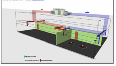
VRML representation of a 3 room model in the VCBT. The data from various building controllers can be shown in real-time.
