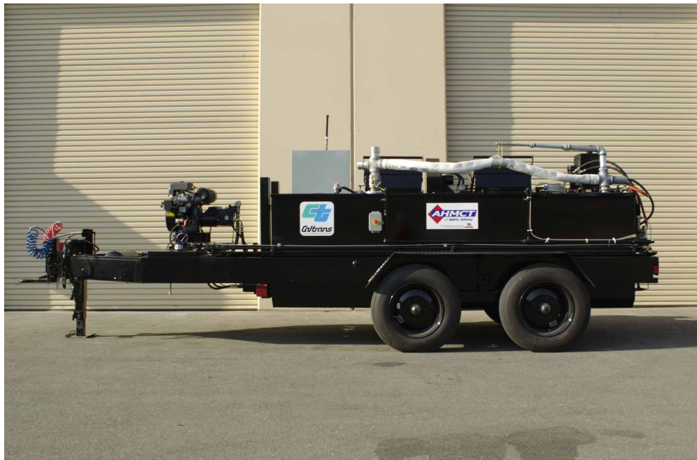
Figure 2 – The Sealant Transfer Tank Trailer – Used to re-supply the Sealzall application truck kettle with large amounts of hot sealant as a method of further increasing highway seal production rates.
