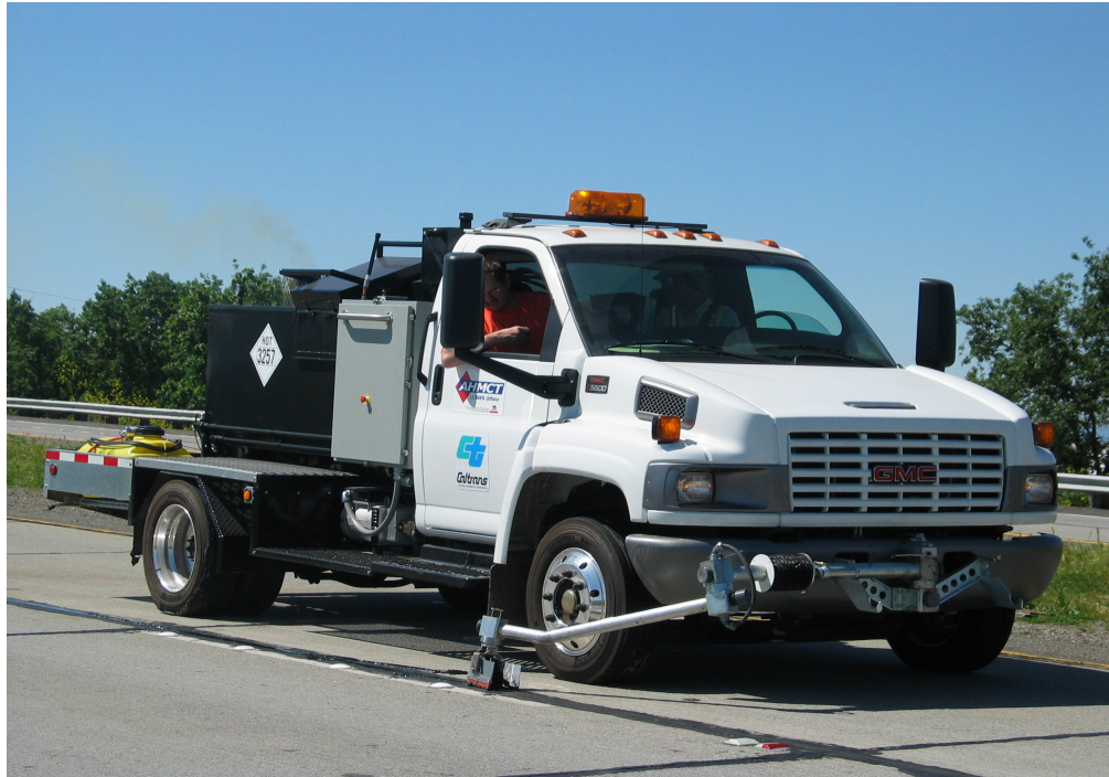
Figure 1 – Sealzall Machine - Automated High Production Longitudinal and Manual In-Lane Crack Sealing
