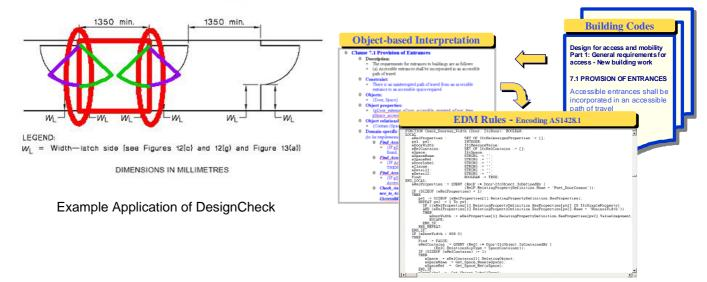
Building codes are interpreted into object-oriented representation and then encoded into rules
