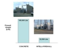
Fig 7. Overall Weight Comparison
