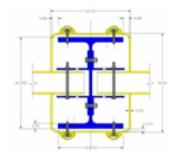
Fig 5 Steel Columns (Blue) CBC Fire Protection Materials (Yellow)
