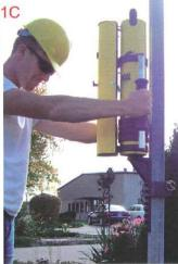
Illustration 1A through 1C on left shows how our side mount adapter works for driving U channel posts. As stated, we offer a full line of both side mount and top mount adapters for driving a full range of posts.
