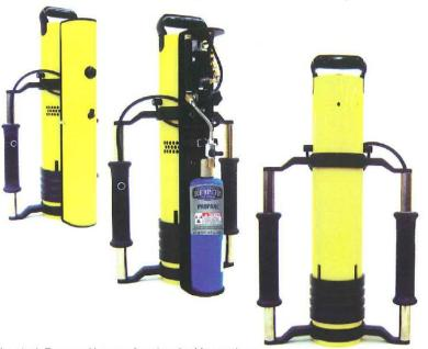
The stock Propane Hammer is set up to drive posts up to 1 5/8" in diameter. You can quickly enlarge the opening to accommodate up to 2 5/8" by removing the ram insert.
