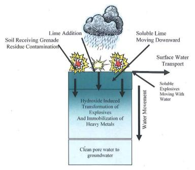
This schematic illustrates the process of alkaline hydrolysis destruction of explosive residues. Rainwater wets the soil that contains the lime. The chemical reaction occurs in the soil pore water resulting in a chemically reactive zone that prevents migration of the explosives into the groundwater. Lime on the surface of the soil prevents transport of explosive particulates in the runoff water.
