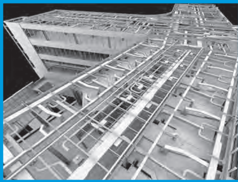
Building Information Model (BIM) of the MEP corridor racks
