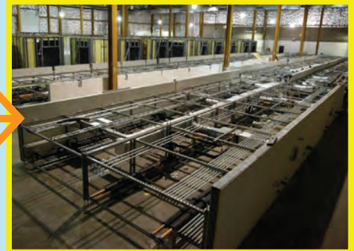
MEP corridor racks lined in the prefabrication warehouse
