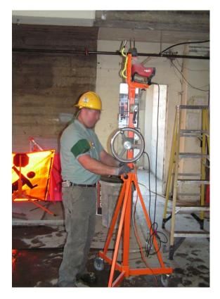
Figure 3: Overhead drill press in the field
