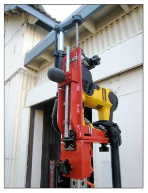
Figure 1: Details of saddle with dustcapturing drill installed
