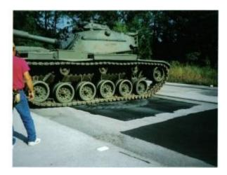
M60-Tank Performs 360 Turns on E-Krete<sup>®</sup> Surface Demonstrating E-Krete<sup>®</sup> Durability
