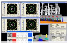
Screenshot of 3D computer model visualization to safely and accurately place concrete shells on river bottom despite flowing and muddy river.
