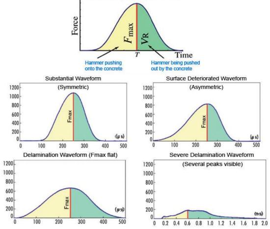
Schematic Diagrams showing general waveform and forms for strong and weaker/deteriorated concrete Construction Innovation Forum • 6494 Latcha Road, Walbridge, OH 43465 • 419-725-3108 • Fax: 725-3079 • E-mail: info@CIF.org • www.CIF.org
