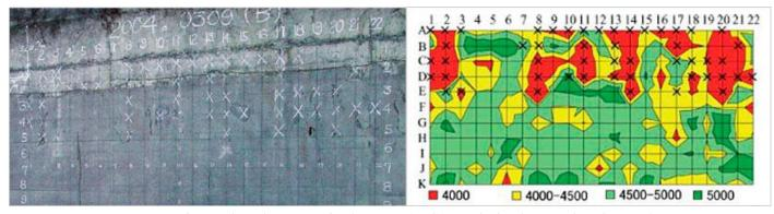
X represents points evaluated as poor using hammer. A PC can calculate hammer based strength contours Schematic Diagram of Impact Waveform
