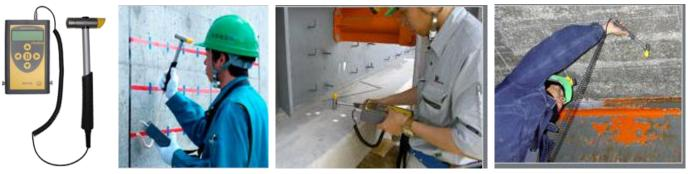
Tester apparatus and testing for strength, deterioration, and delamination
