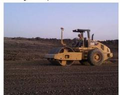
Shown is NorthGate equipment utilizing the intelligent compaction software, with the receiver at the top.
