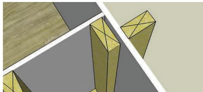
Offsetting the interior wall framing from the exterior wall framing allows drywall to be slid between the two rather than stopping at each corner so the drywall can form a continuous air barrier along the exterior wall.
