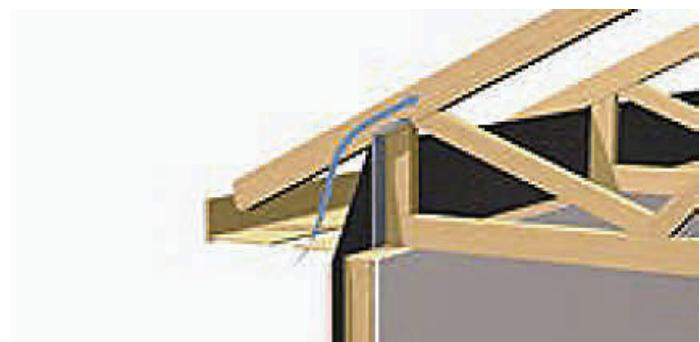
When OSB or plywood wall sheathing is extended up the wall, it provides adequate support for raised heel trusses so no extra blocking is needed. The sheathing also serves as an insulation baffle.
