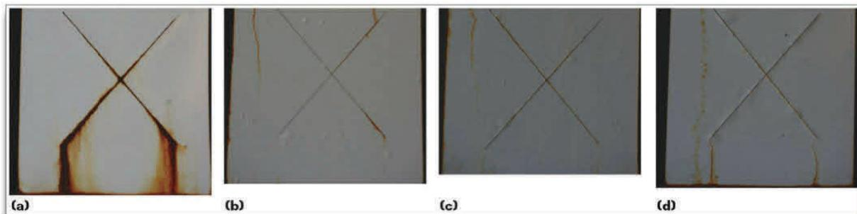
Coupons showing typical three-coat zinc-rich coating system (a) vs two-coat zinc primer nanocoating and three different topcoats (b, c, d) after 5,000 hr exposure in ASTM B117 salt spray (fog) test.
