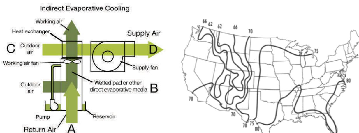
In the figure return air (A) from the space and outdoor air pass directly over a wetted medium (B) to passively remove sensible heat through DEC and then pass through the heat exchanger and is discharged. Outdoor air (C) enters as a supply air stream, passes through the heat exchanger and is 'indirectly' evaporatively cooled before being delivered to the space (D). Compressor-based equipment can be stage-2 cooling following D.
